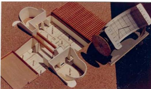
▲ *The schematic design phase sometimes includes a rough cardboard model. For the Kirchner Residence, Queen Creek, AZ, a "Shade Dial" device is simulating solar angles and shading for winter and summer conditions.*
